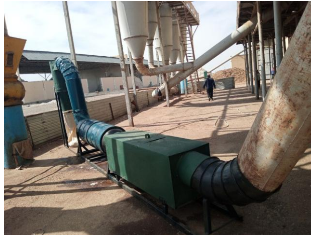
Figure 5. General view of the recommended dust air cleaning device in the pre-cyclone process of cotton pre-processing
