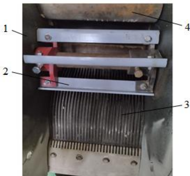
1- working camera, 2- improved blades , 3- saw cylinder, 4- density valve .
