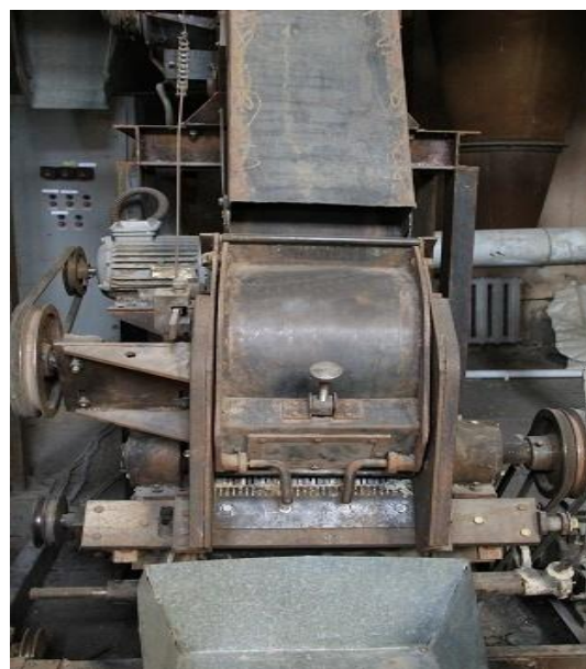
Picture 2. Improved view of a 30 saw 5LP linter with an agitator.
